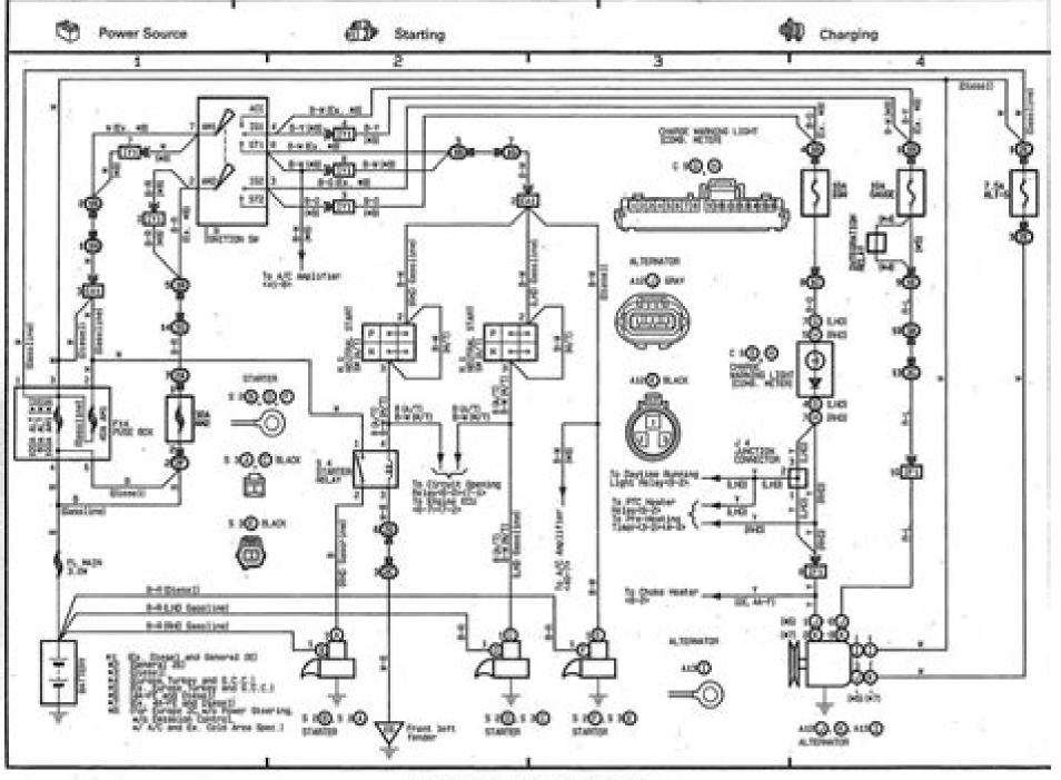
Wiring diagram for charge and start
