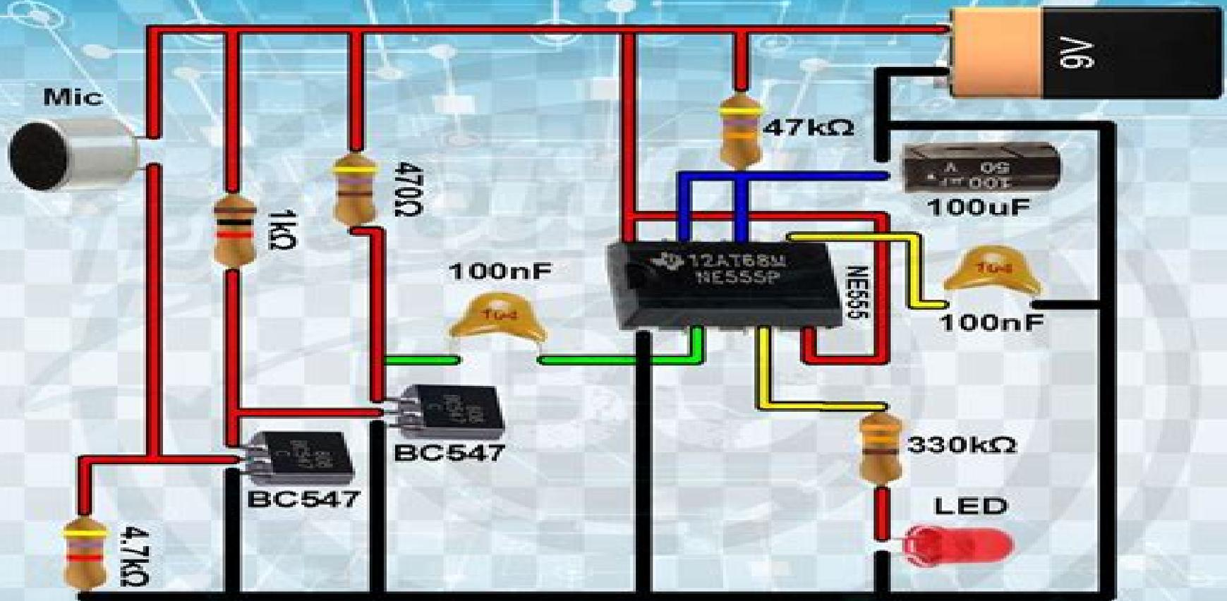
**Clap Switch Circuit Diagram**
