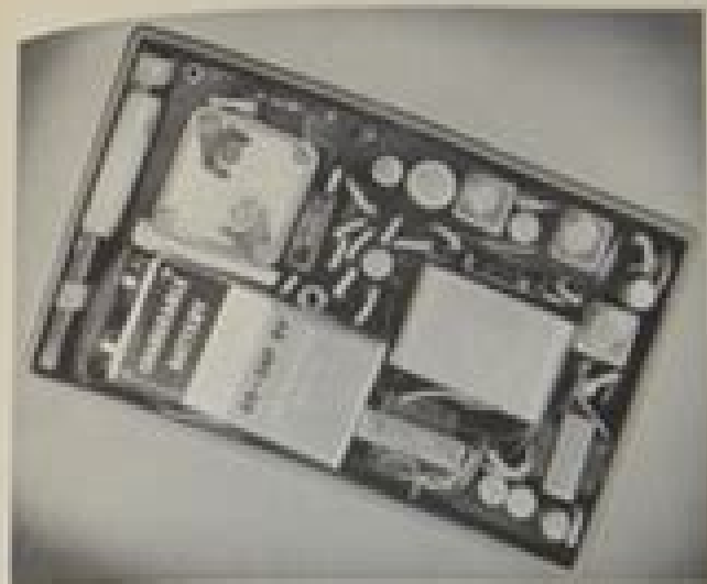
Fig. 425. Circuitry for six transistors fits compactly in the same space used by the receiver in Fig. 424.
