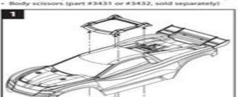
Remove the existing roof skid plate.
