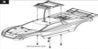
install the new roof skid plate; feed the wire harness. connector through the hole in the roof.
