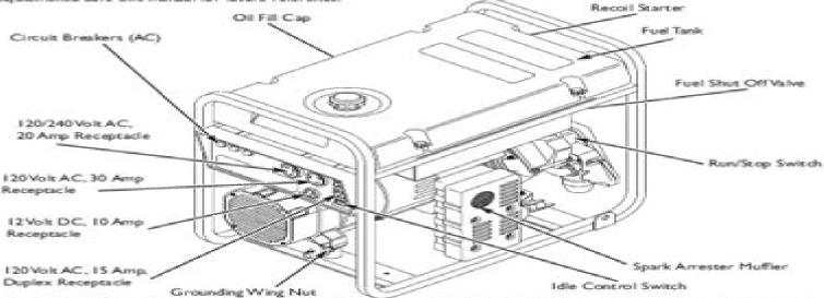
12 Volt DC, 10 Amp Receptacle — Use this receptacle with battery charge cables to charge a 12 Volt battery.
