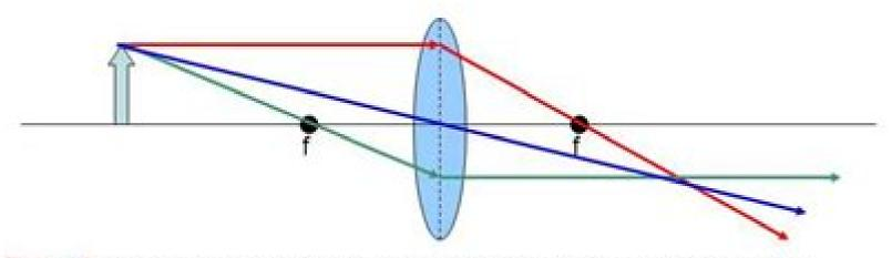
Rule #1: Draw a ray, starting from the top of the object, parallel to the principal axis, then through "f" after refraction.
