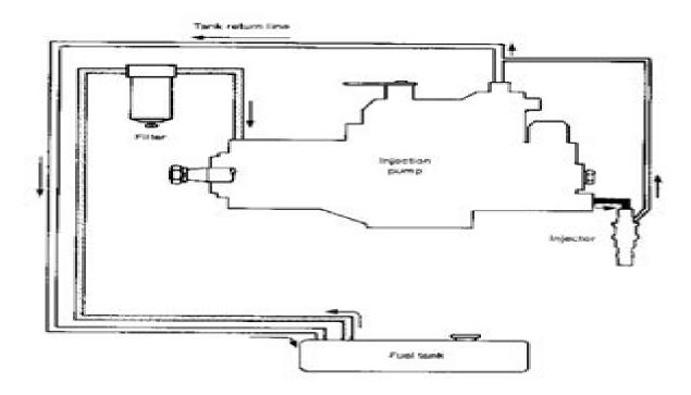
Diesel fuel is drawn from the fuel tank through the filter by the injection pump.
