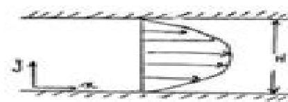
note, Pressure drops in the direction of flow,  $\frac{dp}{dx} < 0$  in velocity equation.
