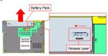
White Release Lever is slid in the left, remove the Battery Pack.
