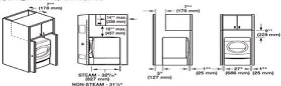
"Required spacing: "For side or bottom venting, 2" (51 mm) spacing is allowed.
