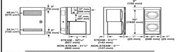
For cabinet installation, with a door, the minimum ventilation openings in the top are required.
