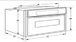
A. 26 Nr (71.2 cm) max, recessed width 8. 29" (73.7 cm) max, overall height C. 29 Nr (75.6 cm) overall width D. 23" (58.4 cm) max, recessed depth
