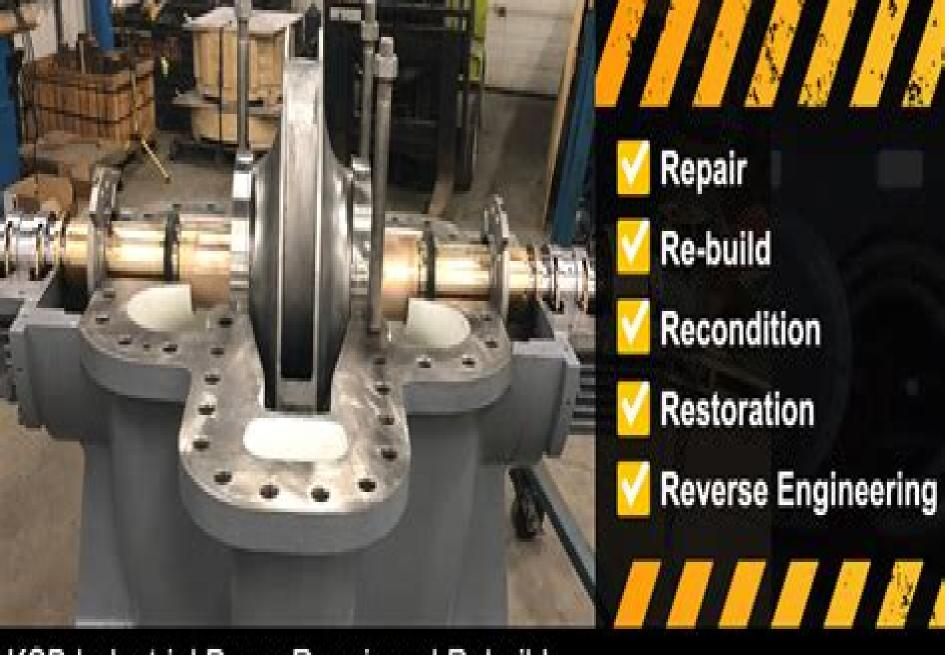
KSB Industrial Pump Repair and Rebuild
