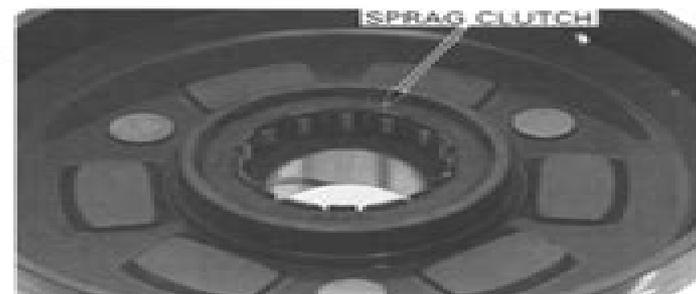
Remove the sprag clutch from the clutch outer. Check the clutch lining and sprag clutch contacting surfaces for abnormal wear or damage.
