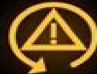
TRACTION CONTROL MALFUNCTION
