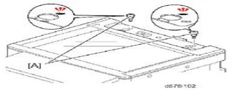
2. Insert the two stud screws [A] on the top of the machine.
