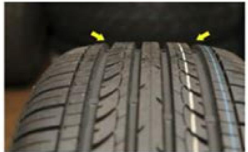
Puncture repairs are limited to the center of the tread area. If there are punctures or damage in the shoulder or sidewall of the tire, it is not repairable.
