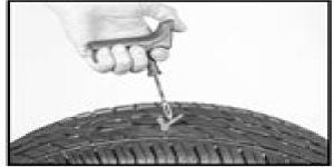
Pull the plugger tool straight out of your tire with a rapid motion, leaving the tire plug behind. Do not twist the needle.
