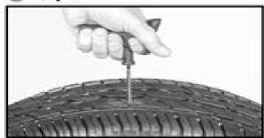
Slide the reamer tool in and out of your tire puncture multiple times to roughen and clean the inside of the hole.
