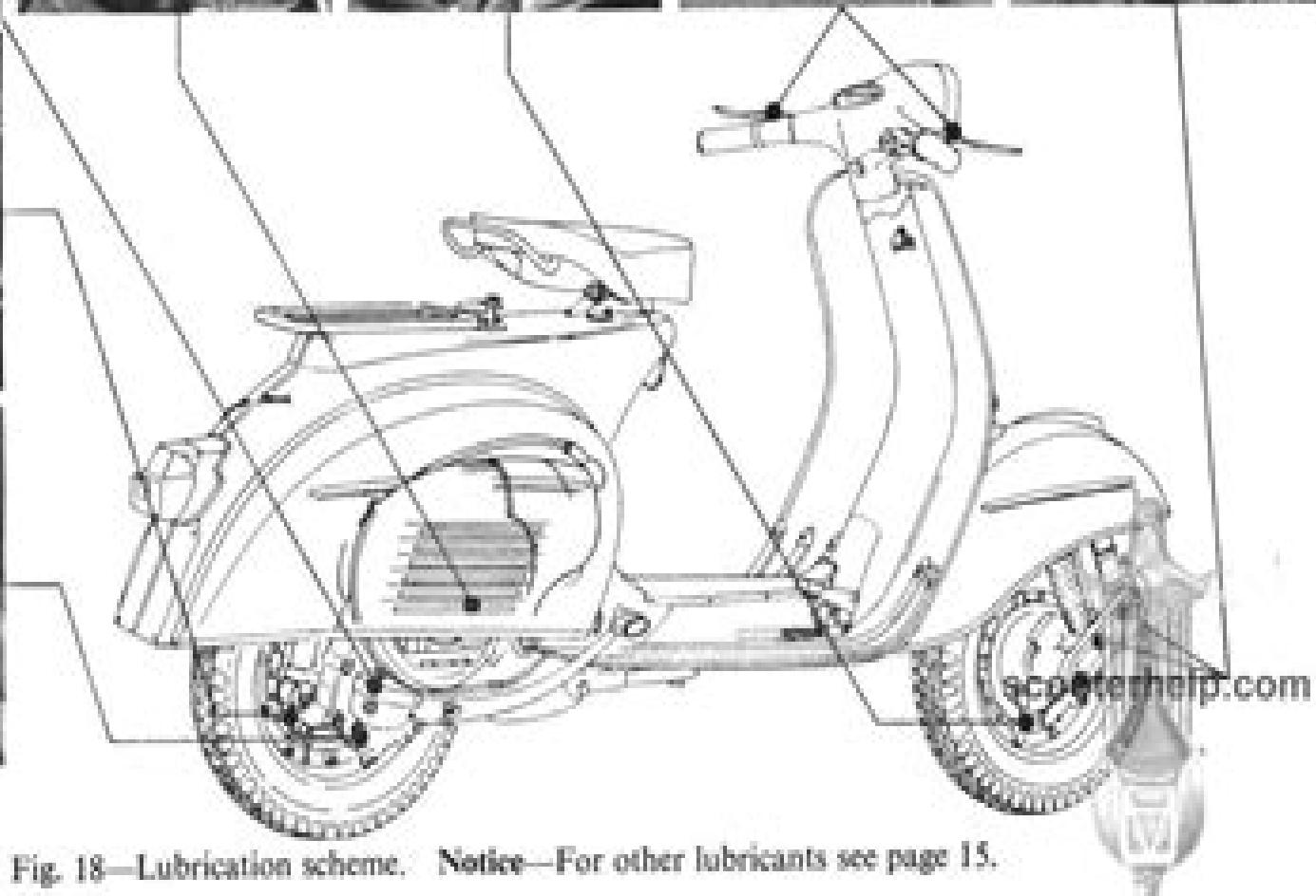
Fig. 18—Lubrication scheme. Notice—For other lubricants see page 15.
