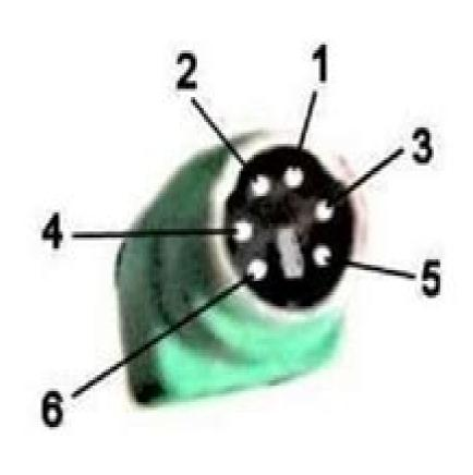
louse connector pinout is identical to PS/2 keyboard.
