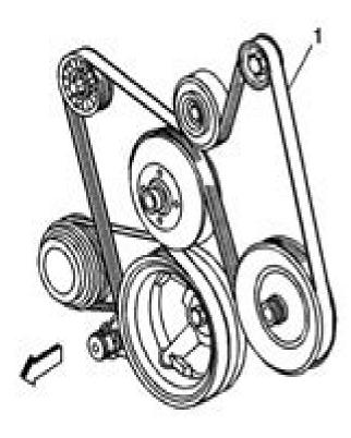
Fig. 2: View Of Drive Belt (LSL, S.JL, and 6.0L Engines) Courtesy of GENERAL MOTORS CORP.
