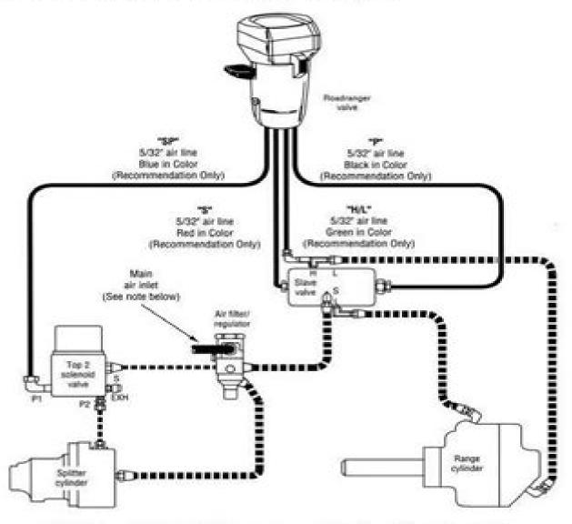
NOTE: Main air inlet is 1/4' I.D. hose connected to either of the main air tanks.
