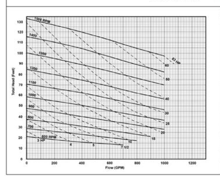
Suction: 4" Discharge: 4" Impeller Dia: 15-7/6" Max Sphere Size: 4.0"
