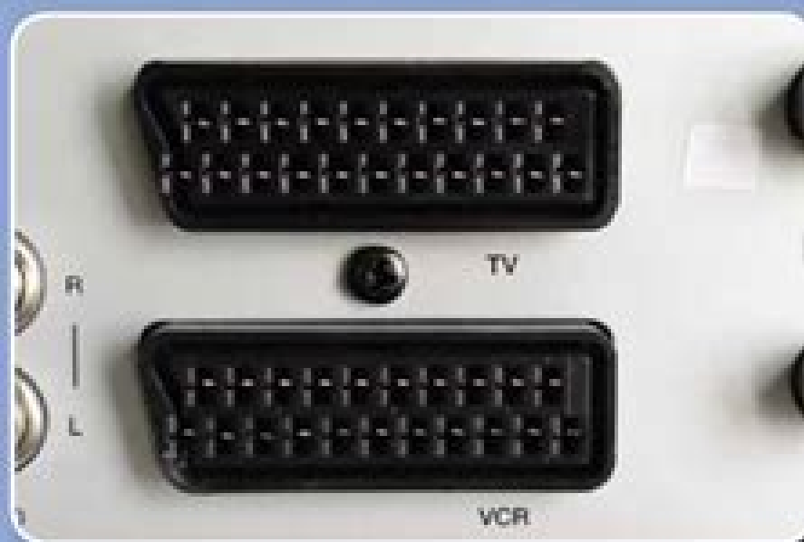
Common with European receivers: the two SCART plugs for connecting TV and VCR
