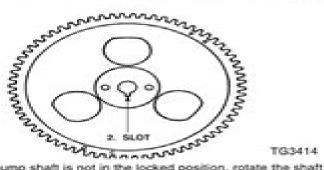
If the pump shaft is not in the locked position, rotate the shaft clockwise until the key on the shaft and the slot in the drive gear are aligned.
