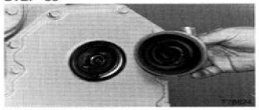
Install the tachometer drive assembly (if equipped).
