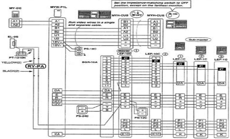
The BGR-10A Music Control Center provides the All Call, Door Chime, and Radio features. For receiving a chime from the door and making an all call from the LEF-1C stations, the BGR-10A is required in the system.
