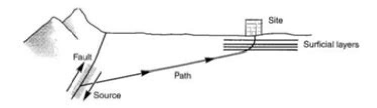
Assumption: all the boundaries are horizontal and the response of a soil deposit is predominantly caused by SH-waves propagating vertically from the underlying bedrock.
