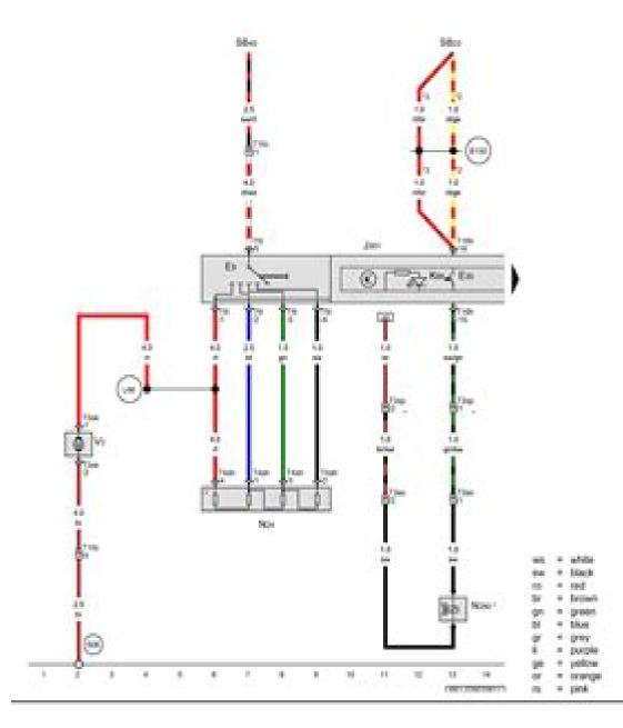
Fresh air blower switch, Air conditioning system control unit, Fresh air blower series resistor with overheating fuse, Fresh air blower
