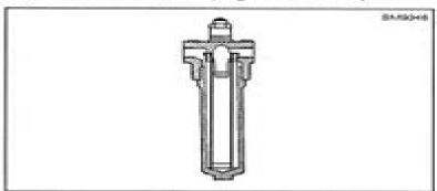
Type: Hydraulic Oil Filter (High Pressure) is a main system filter that contains a magnetic particulate plug in the upper casting.
