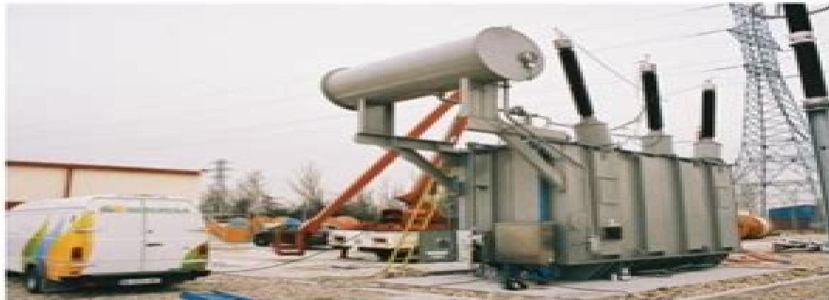
FIG. 2. Field testing of a power transformer before putting into service (SOMINA).
