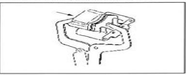
NOTE: Brake fluid will be forced through compensating port into master cylinder fluid reservoir when piston is pushed back into caliper. Remove excess fluid from reservoir as required.
