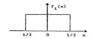
$$\underline{\xi}(\omega) = \left[\frac{2\sin(\omega/2)}{\omega}\right]^3 = \left(1 - \frac{\omega^2}{24} + \frac{\omega^4}{1920} - \cdot \cdot\right)^3$$
