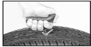
With the plug centered in the eye of the needle, start pushing the plugger tool and plug into your puncture. Stop pushing when the plug is 2/3 of the way into the hole.
