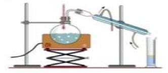
In distillation, the mixture of liquids begins in an initial flask. It is heated until one of the liquids evaporates away. The gaseous substance is then cooled and returns to the second flask as a liquid.
