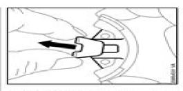
Pull the retainers, if fitted, off the clutch shoes.
