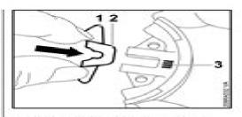
On retainers with tabs (1), the narrow side (2) must be next to the series number (3).
