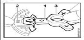
Fit the clutch shoes over the arms (1) of the clutch carrier so that the series number (2) is on the same side as the larger hexagon (3).
