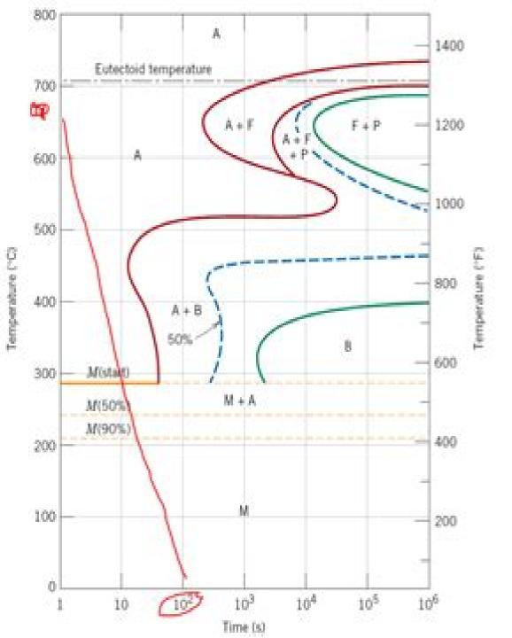
Figure 10.23 Isothermal transformation diagram for an alloy steel (type 4340): A, austenite; B, bainite; P, pearlite; M, martensite; F, proeutectoid ferrite. [Adapted from H. Boyer (Editor), Atlas of Isothermal Transformation and Cooling Transformation Diagrams, American Society for Metals, 1977, p. 181.]
