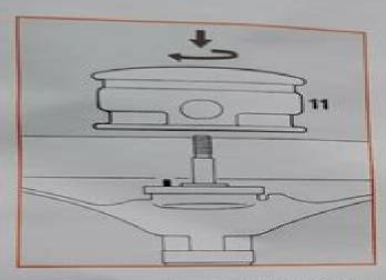
Screw mowing head (11) clockwise onto the shaft as far as it will go and tighten down firmly.
