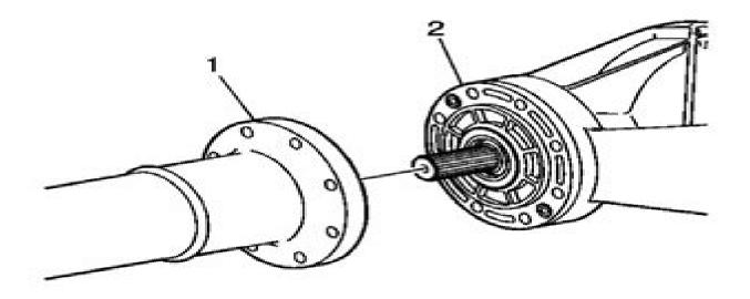
Fig. 12: View Of Torque Tube & Differential Pinion Shaft Courtesy of GENERAL MOTORS CORP.
