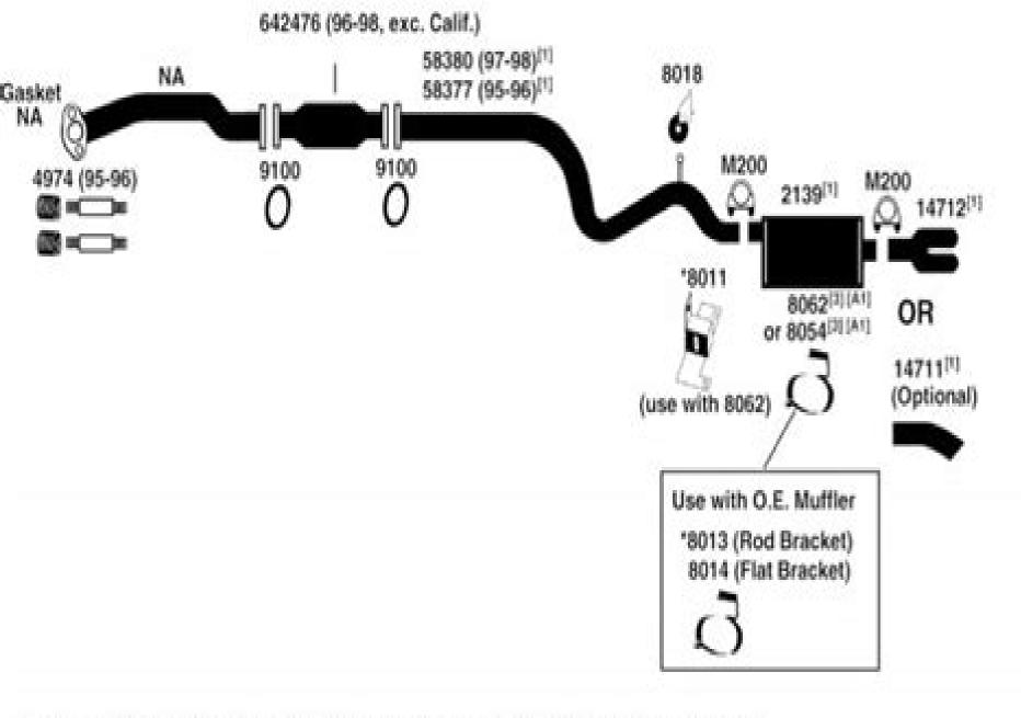
[A1] Use 8062 for Muffler Strap w/flat bracket. Use 8054 for Muffler Strap w/rod bracket.
