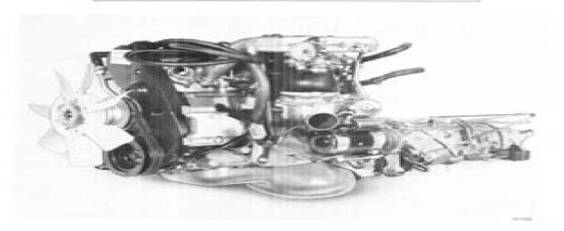
Prior to removing, coolant and engine oil must be drained. Distributor cap on rearmounted distributor must be removed.
