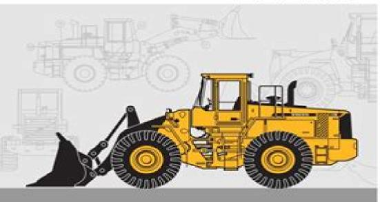
Engine output SAE J1995; power, gross 259 kW (352 hpl) 15/0 9249, SAE 21349: power, net 297 kW (349 hpl)
