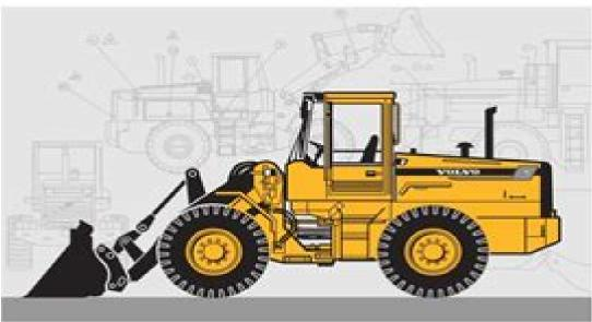
Engine output SAE /1349: gross 96 kW (130 hg) net 90 kW (122 hg)
