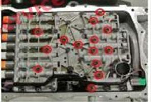
11. Using the utmost care, lift the mechatronic symmetrically, then nemove it from its seat on gearbox.
