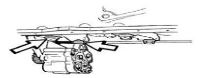
Remove the bolts for the front main bearing cap and lift down the lubricating oil pump together with the main bearing cap.
