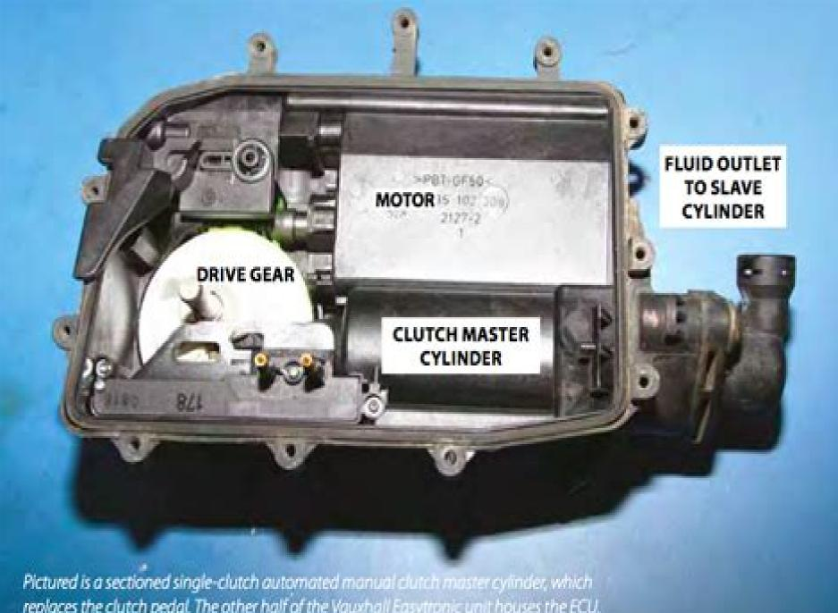
replaces the clutch pedal. The other half of the Vauxhall Easytronic unit houses the ECU.
