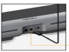
Be sure to remove the protective caps from each end of the optical audio cable before inserting.
