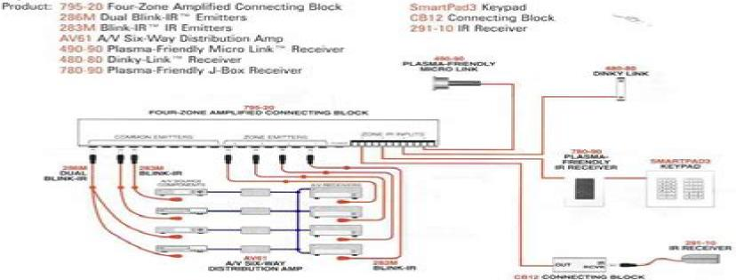
7. MULTI-ROOM SINGLE-ZONE BACKGROUND MUSIC SYSTEM for custom residential or commercial applications. Provides independent room volume control via IR using PA1235-12-Channel Power Amplifier with built-in IR control and IR controlled music source such as a CD changer or digital music source, eliminating the need for a multi-room preamp.
