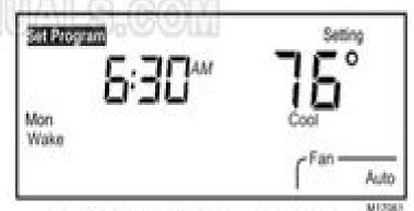
By pressing Increase v or Decrease w, you select the cooling Wake temperature. Example display shows the cooling Wake period set for 76'r.
