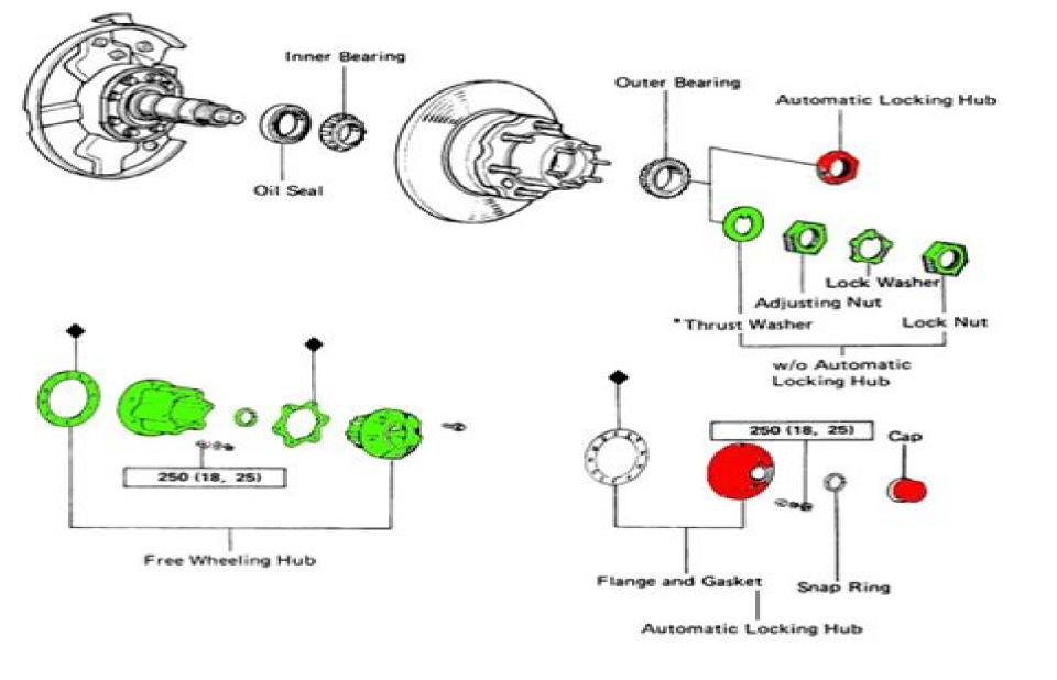
CAUTION: When converting to an automatic locking hub from a hub without free wheeling hubs or a free wheeling hub, a thrust washer must not be installed.
