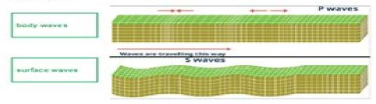
P-waves and S-waves are seismic waves that move through the earth's interior. On the
