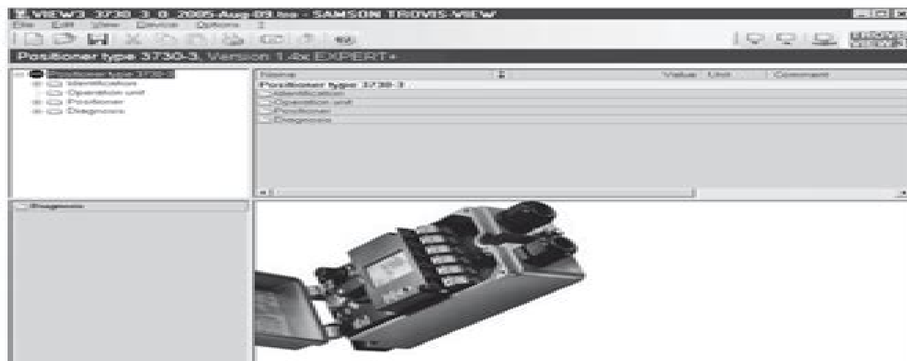
Fig. 1 - Valve diagnostics with SAMSON TROVIS-VIEW Operator Interface, e.g. for Type 3730-3 Positioner
